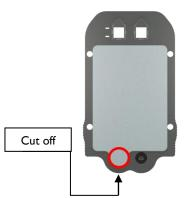
2. Pipette a minimum of 200 µl of sample / positive control into the open sample well on the right as indicated below.
